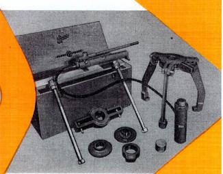
Flexi-Force equipment does not have to depend on any outside power source—although motorised pumps are available if required for repetitive work. It is relatively portable and invariably can be taken to the job.
